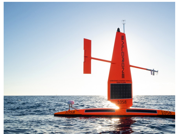
Figure 3: The Danish navy has developed autonomous "saildrone" that can remain months at sea.
